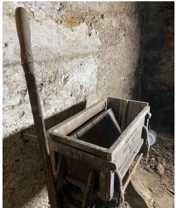
Photo of brick-making machine used by students to make bricks for building Koren, 2021. (Taken by Uwe Rudolf)
